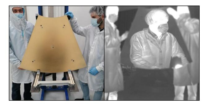
The gold-colored ASTHROS mirror panels appear blurry to the naked eye, as seen at left. But when photographed with an infrared camera, as at right, the panel reflects a technician's image as clearly as if the person were looking in a mirror. Credit: Media Lario
