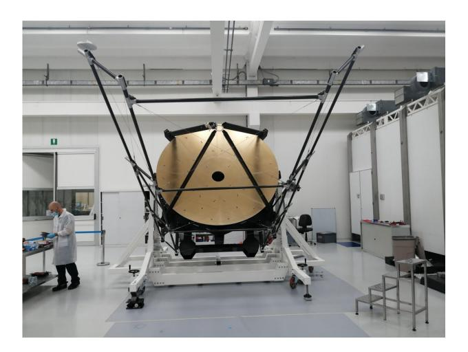
The ASTHROS mission's primary mirror is one of the largest to ever fly on a high-altitude balloon. The lightweight mirror is coated in gold and nickel to make it more reflective in far-infrared wavelengths. Credit: Media Lario
