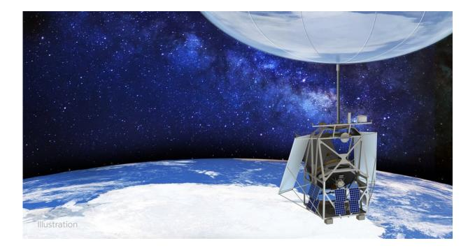
Lofted by a stratospheric balloon, as shown in this illustration, NASA's ASTHROS mission may reach an altitude of 130,000 feet (40 kilometers). From that height, the telescope can detect wavelengths of light that are blocked by Earth's atmosphere and cannot be observed from the ground. Credit: NASA/JPL-Caltech
