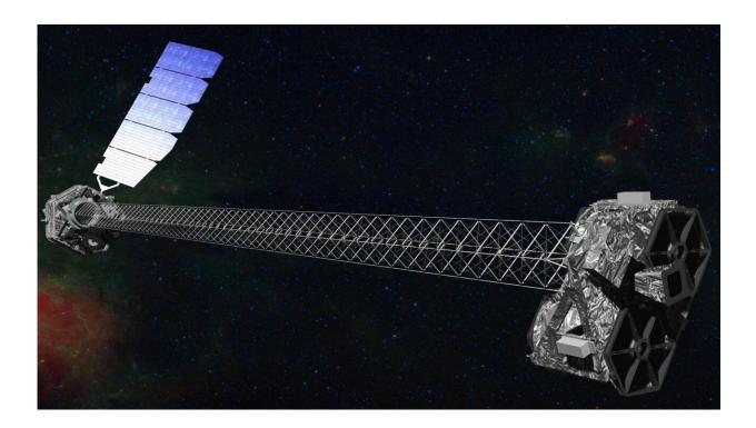
NASA's NuSTAR space telescope, shown in this illustration, features two main components separated by a 30-foot (10-meter) mast, sometimes called a boom. Light is collected at one end of the mast and is focused along its length before hitting detectors at the other end. Credit: NASA/JPL-Caltech
