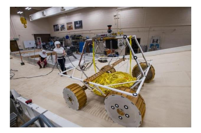
A prototype of the VIPER moon rover is tested in the Lunar Operations Lab. Credit: NASA
