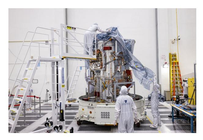
Engineers and technicians unwrap and inspect the main body of NASA's Europa Clipper spacecraft after it was built and delivered by the Johns Hopkins Applied Physics Laboratory (APL) in Laurel, Maryland, to the agency's Jet Propulsion Laboratory in Southern California. Credit: NASA/JPL-Caltech/Johns Hopkins APL/Ed Whitman
