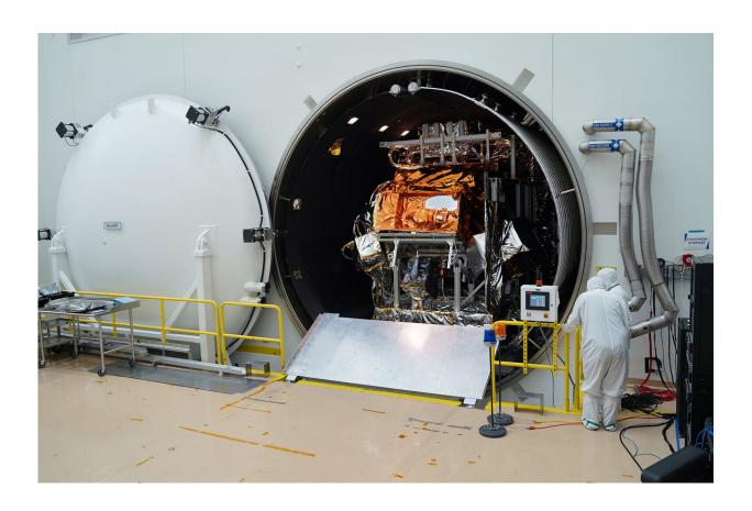
The JPSS-2 satellite enters the chamber for its thermal vacuum test at the Northrop Grumman facility in Gilbert, Arizona. Credit: Northrop Grumman
