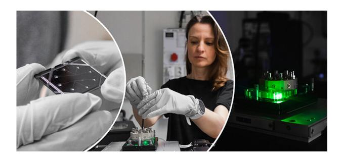
New microscopy method. The biomolecules the researchers want to study are placed in a chip consisting of tiny nano-sized tubes—nanochannels. Test fluid is added to the chip, which is mounted in an optical dark-field microscope and illuminated with visible light. The molecule appears as a dark shadow moving freely inside the channel on a screen connected to the microscope. Credit: Envue Technologies | Maja Saaranen
