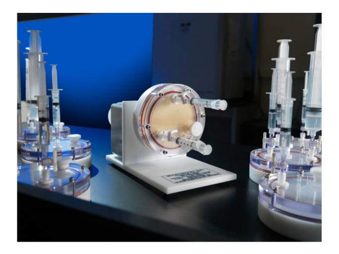
A device known as a RWV (rotating wall vessel) bioreactor was used to simulate the conditions of microgravity encountered by cells during spaceflight missions. Credit: The Biodesign Institute at Arizona State University
