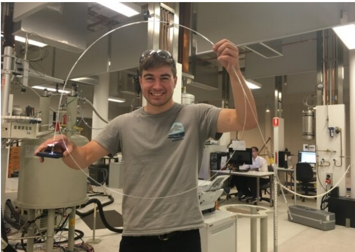
Mr James Watson holding the apparatus used to photolyse (use light to disintegrate) the sample whilst inside the NMR spectrometer. Credit: University of New South Wales
