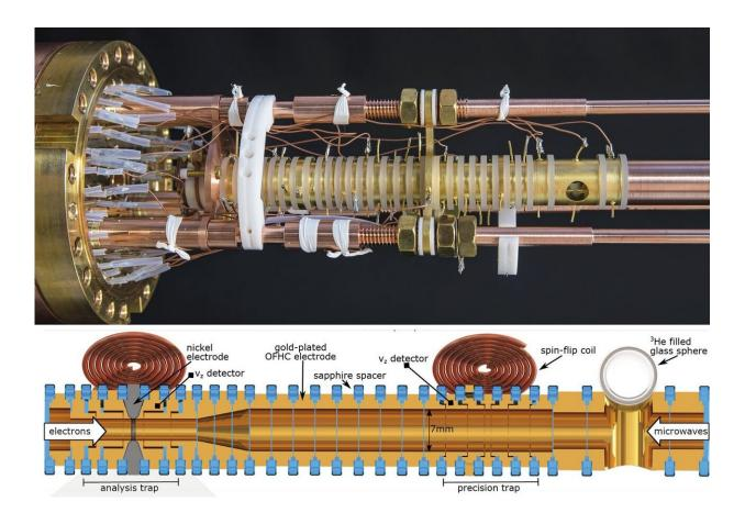
Fig. 2: Photograph and schematic view of the Penning trap for the <sup>3</sup>He<sup>+</sup> hyperfine structure measurement. Credit: MPI
