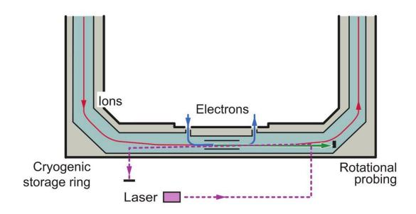
Simplified schematic of the experiment showing the relevant parts of the cryogenic storage ring (CSR). The red and blue trajectories highlight the ion and electron beams, respectively. The stored ions can interact with the merged electron beam or a pulsed laser beam (dashed purple line). The laser interaction products are neutral and continue ballistically (green arrow) until collected on a particle counting detector. Credit: Kalosi et al.
