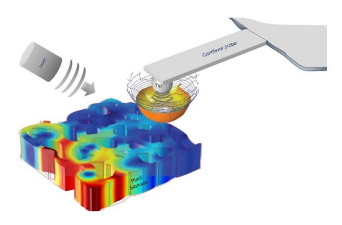
Scattering-type scanning near-field optical microscopy, a nondestructive technique in which the tip of the probe of a microscope scatters pulses of light to generate a picture of a sample, allowed the team to obtain insights into the composition of plant cell walls. Credit: Ali Passian/ORNL, U.S. Dept. of Energy
