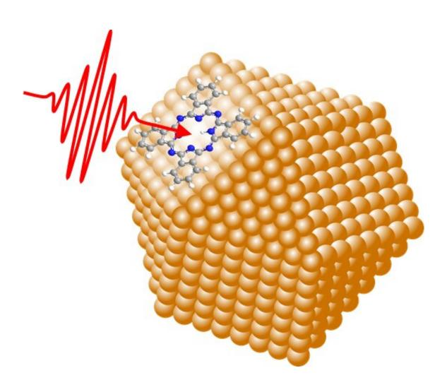
Laser excitation of a phthalocyanine molecule on the surface of a noble gas cluster consisting of a few hundred neon atoms. The system has a size of less than ten nanometers. Credit: Ulrich Bangert et al
