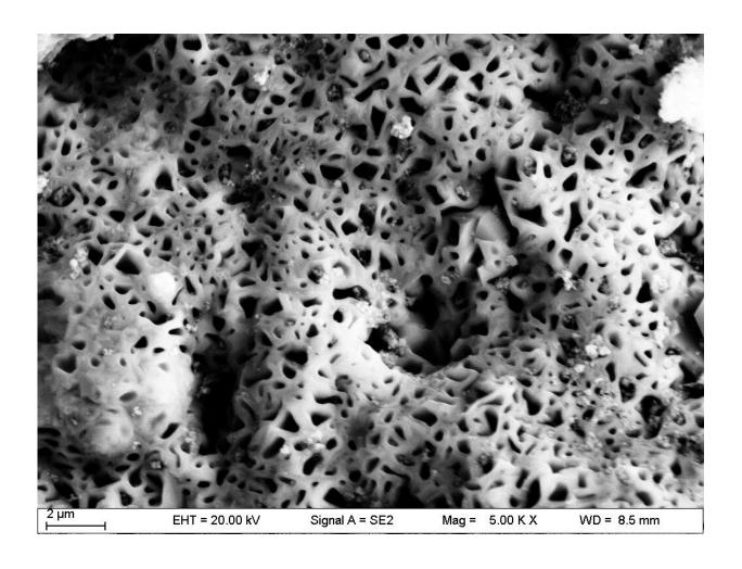
Honeycomb structures in localized regions at the top of the magnetite layer on a martensitic steel after corrosion in LBE. Credit: Luo Lin
