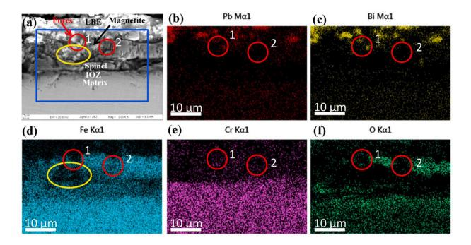
(a). Cross-sectional morphology of steel exposed to LBE containing 10-7 wt% oxygen for 2,000 hours; (b)-(f). Energy Dispersive Spectroscop map scanning results of the area indicated by the blue box in (a). Credit: Luo Lin
