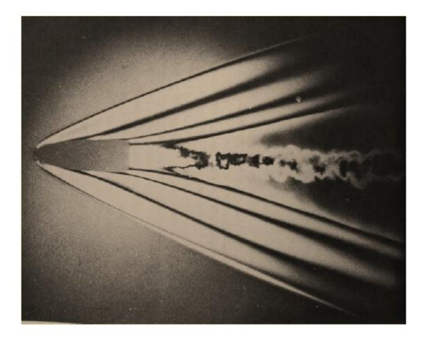
By accident, the laser fired a double pulse, the first of which occurred before the bullet was in the field of view. Credit: Karl A. Stetson
