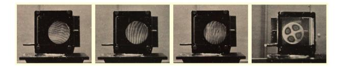
The last two images show the object's vibration as seen in real-time and as a hologram reconstruction. Credit: Karl A. Stetson
