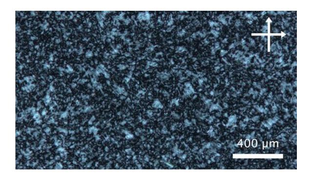
Liquid crystals of boron nitride nanotubes are easy to extrude into fibers through a process developed at Rice University. The fibers could be useful for aerospace and electronics applications and as energy-efficient materials. Credit: Pasquali Research Group
