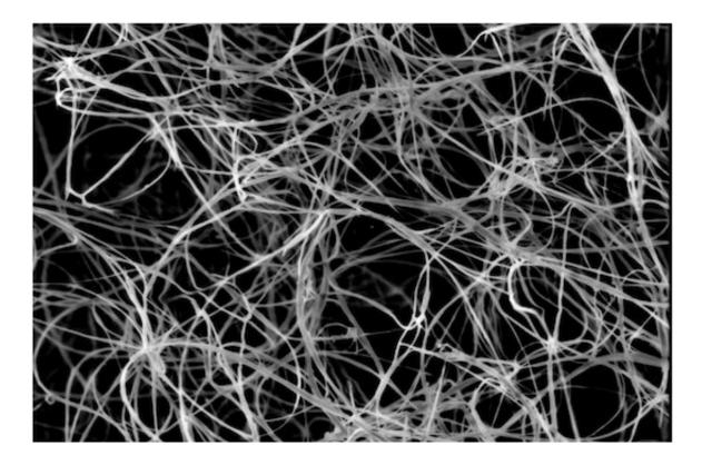
A tangle of unprocessed boron nitride nanotubes seen through a scanning electron microscope. Rice University scientists introduced a method to combine them into fibers using the custom wet-spinning process they developed to make carbon nanotube fibers. Credit: Pasquali Research Group
