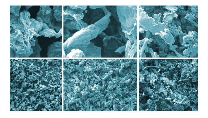
Graphene Flagship researchers analyzed the effect of particles derived from polyamide reinforced with reduced graphene oxide. Colored SEM images of abraded particles. Credit: Empa / *Journal of Hazardous Materials*
