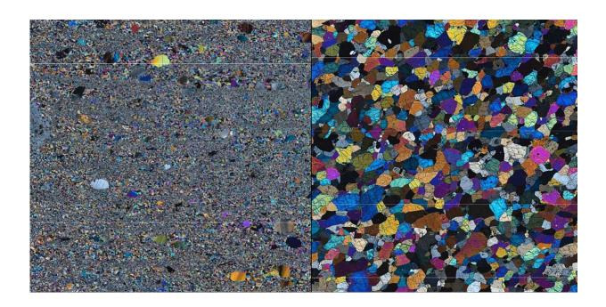
Depending on how coarse-grained the rocks in the upper mantle are, they deform quite differently under stress. The picture shows two microscopic thin sections of mantle rocks. Credit: Jonas Ruh / ETH Zurich
