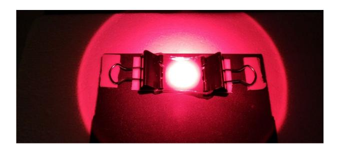
In this experiment, the gel is being activated by a red LED before the researchers measure the light it transmits. Credit: Joonas Ryssy
