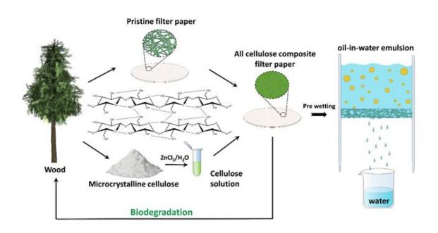
The closed loop process of the degradable cellulose oil-water separation membrane. Credit: Institute of Coal Chemistry (CAS)
