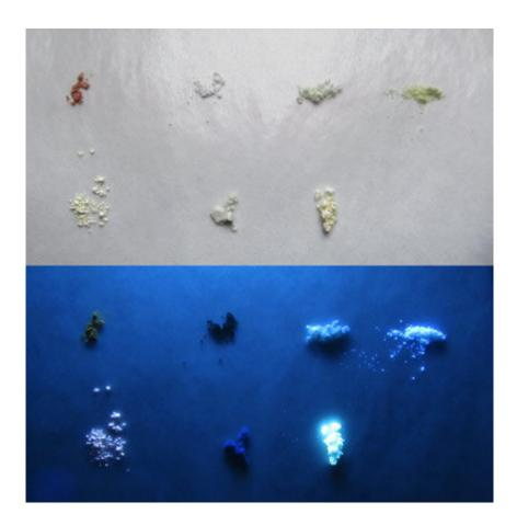
Eight compounds were predicted to fluoresce by a new method for designing molecules. Of the eight, six were found to fluoresce under ultraviolet light (five shown; C, D, E, F, G), including one compound that hadn't been previously reported (not shown). Credit: M. Sumita et al. Distributed under a <u>CC BY-4.0</u> <u>License</u>
