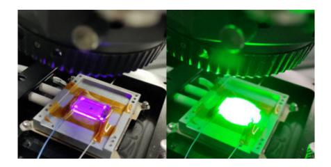
Shining blue light (left) on the fluid caused it to switch to a high dielectric permittivity phase, while shining green light on it (right) reversed the change. Credit: H. Nishikawa *et al*, <u>CC BY 4.0</u>
