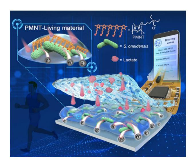
Schematic diagram of PMNT-based living material and bioelectronic device for monitoring lactate in physiological fluids (sweat, urine, and plasma) and counting
