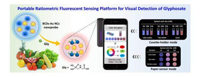
Figure 1. Schematic diagram of the rapid visualization and quantification of glyphosate residues by ratiometric fluorescence sensor. Credit: Zhang Qianru
