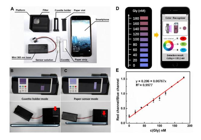
Figure 2. Smartphone-based monitoring platform for visual quantitative detection of glyphosate. Credit: Zhang Qianru
