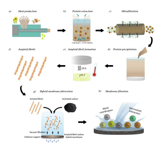
Schematic of process flow from plant seeds to the amyloid-based filtration membrane. a) Production of sunflower and peanut meals by screw-pressing
