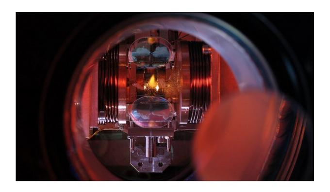
The image shows cold atoms (in yellow) in an optical resonator on their way to form a time crystal. Credit: University of Hamburg
