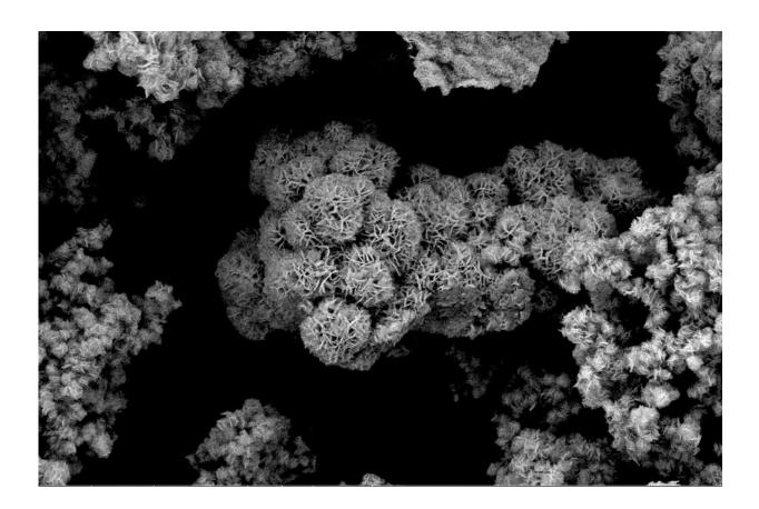
Molybdenum disulfide under the scanning electron microscope. Credit: Vienna University of Technology
