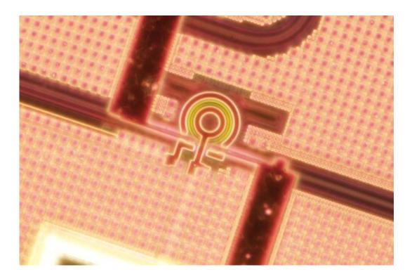
Photonic chip with a microring resonator nanofabricated in a commercial foundry. Credit: Joel Tasker, QET Labs
