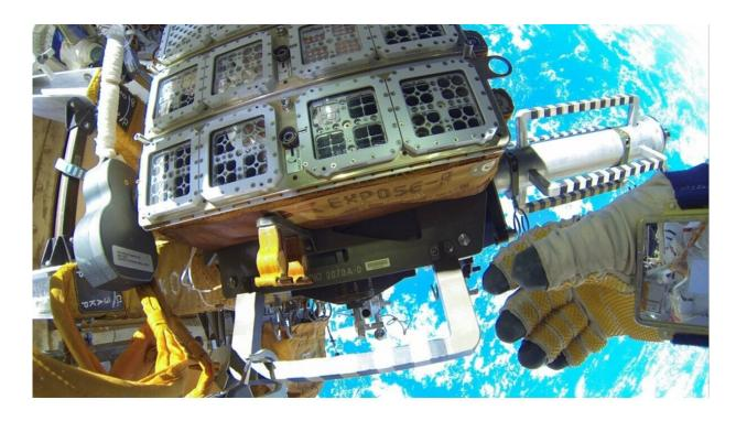
Another platform (EXPOSE-R2) outside the International Space Station (ISS) for simulating a Mars-like environment that was used for the experiments. Credit: European Space Agency (ESA)
