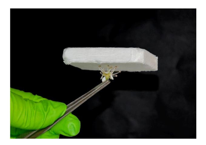
A close-up of the aerogel for insulation, developed from wood cellulose. Credit: Jonas Garemark/Wallenberg Wood Science Center, KTH Royal Institute of Technology
