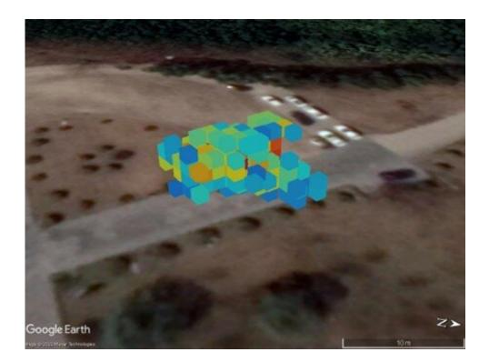
3D image of a leaked gas cloud overlayed on a digital map. The overlay provides detailed information about the leak such as location, volume and concentration, which could be used to provide early warnings, assess risk or determine the best way to fix the leak. Darker red indicates a higher concentration of  $CH_4$  within a cloud. Credit: Yunyou Hu, Anhui Institute of Optics and Fine Mechanics, Chinese Academy of Sciences
