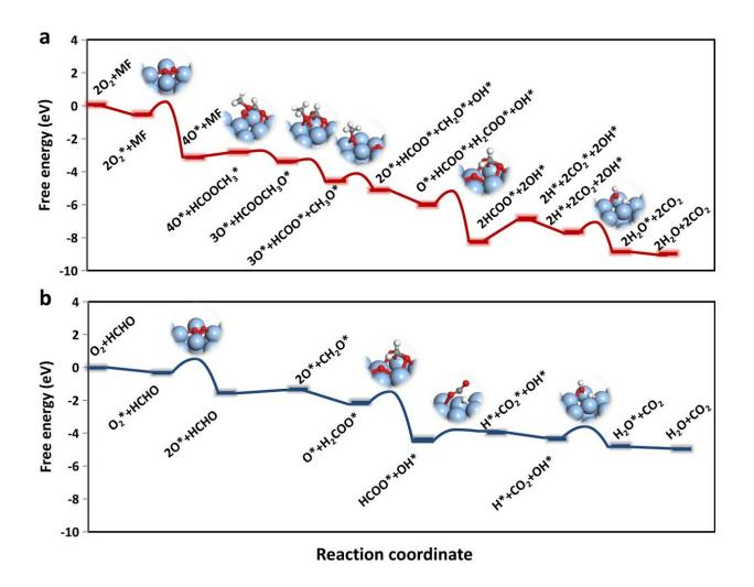
Free-energy diagrams of the oxidation processes. a MF (red line) and b HCHO (blue line) oxidation on Ag(100) surface, respectively. The transition-state structures are shown as insets, where the Ag, C, O, and H are represented in silver, gray, red, and white, respectively. Credit: *Nature Communications* (2022). DOI: 10.1038/s41467-022-29936-8
