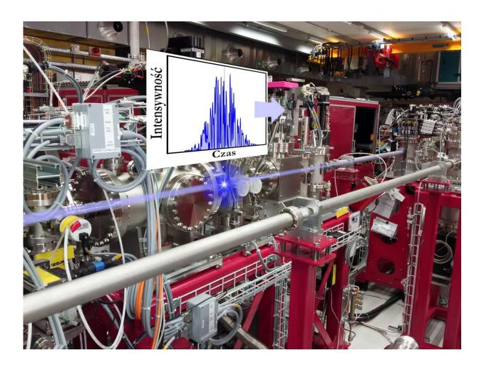
Attosecond phenomena can be studied with free electron lasers such as SwissFEL (the photo presents its research station Alvra). X-ray chronoscopy, which analyzes the shape of laser pulses before and after interaction with the sample, can potentially provide the most accurate image of these phenomena. Credit: Source: IFJ PAN / Paul Scherrer Institut / SwissFEL Alvra
