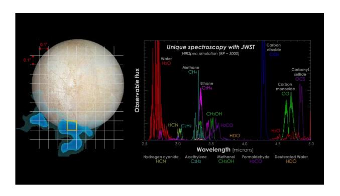
Simulated spectroscopy results from the plumes of Europa. This is an example of the data the Webb telescope could return that could identify the composition of subsurface ocean of this moon. Credit: NASA-GSFC/SVS, Hubble Space Telescope, Stefanie Milam, Geronimo Villanueva
