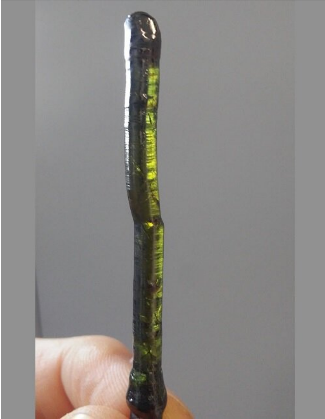
A sample of the frustrated cerium-based magnet, \text{Ce}_2\text{Zr}_2\text{O}_7 , designed in Andrea Bianchi's lab. Credit: University of Montreal
