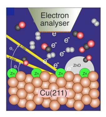
Figure illustrates a Cu surface covered with small amount of Zn probed with photoelectron spectroscopy during reaction of CO2, CO and H2 to methanol. Credit: Stockholm University
