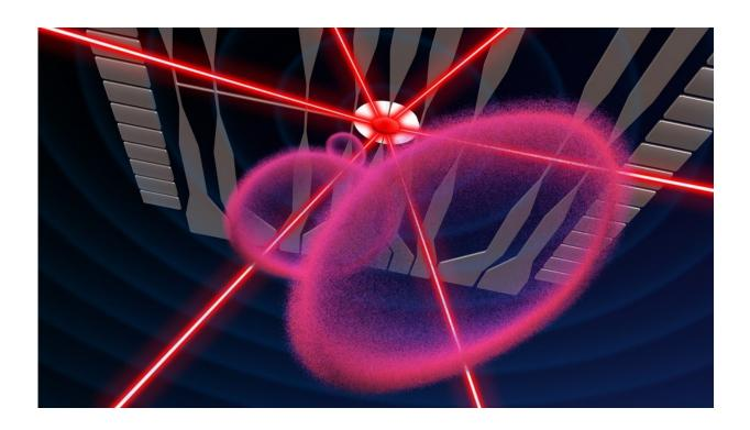
Inside NASA's Cold Atom Lab, scientists form bubbles from ultracold gas, shown in pink in this illustration. Lasers, also depicted, are used to cool the atoms, while an atom chip, illustrated in gray, generates magnetic fields to manipulate their shape, in combination with radio waves. Credit: NASA/JPL-Caltech
