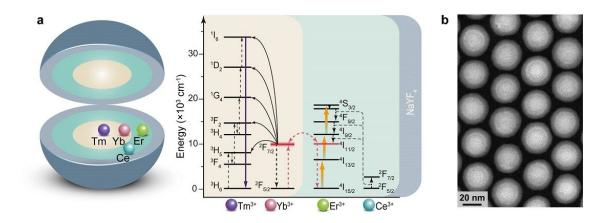
(a) Schematic design of a NaYF4:Yb/Tm@NaErF4:Ce@NaYF4 core—shell—shell nanoparticle for domino upconversion (left panel) and the proposed energy transfer mechanism in the nanoparticle. (b) A high-angle annular dark-field scanning transmission electron microscopy (HAADF-STEM) image of the NaYF4:Yb/Tm@NaErF4:Ce@NaYF4 nanoparticles, highlighting the layered structure. Credit: City University of Hong Kong
