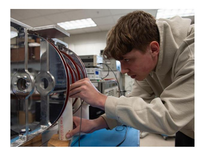
Engineering science and mechanics doctoral student Fedor Sharov adjusts settings in a very low frequency EDMR spectrometer. Credit: Kelby Hochreither/Penn State
