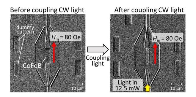
The researchers demonstrated light-induced thermomagnetic recording for the first time. The magnetic direction changes direction after light is coupled into the magnetic area of the CoFeB magnetic film on the silicon waveguide. Credit: Toshiya Murai, Tokyo Institute of Technology
