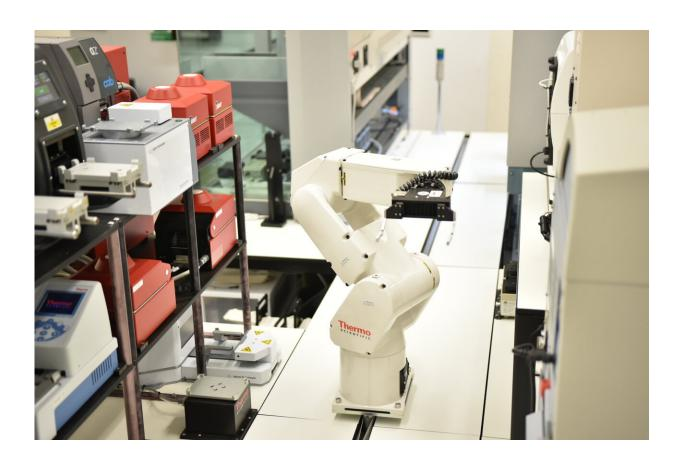
The Illinois Biological Foundry for Advanced Biomanufacturing (iBioFAB) supports the automated construction of plasmids through a new platform called PlasmidMaker. Credit: CABBI
