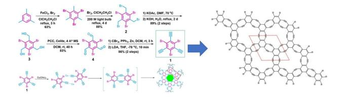
Holey graphyne (HGY) produced using bottom-up synthesis. The molecular structure of HGY is highly consistent with alternately linked benzene rings and C≡C bonds, comprised of six-vertex and highly strained eight-vertex rings and an equal percentage of sp2 and sp hybridized carbon atoms. Credit: Institute for Basic Science
