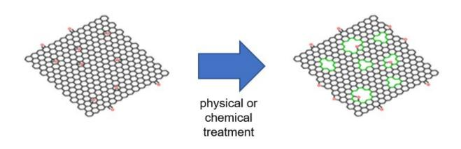
Holey graphene produced using a conventional top-down approach. The size and distribution of holes generated are uneven. Credit: Institute for Basic Science
