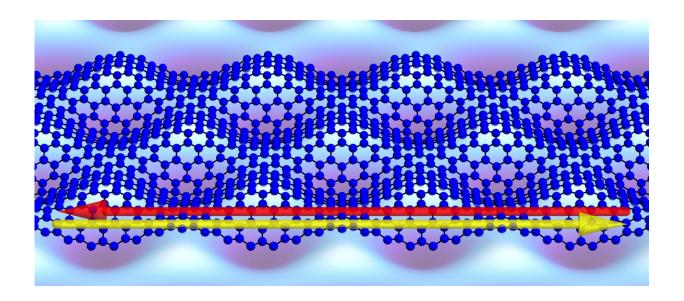
A depiction of a carefully-designed substrate that causes a deposited sheet of graphene to ripple. This distortion generates currents that reside on only one side of the nanoribbon structure. Credit: Võ Tiến Phong
