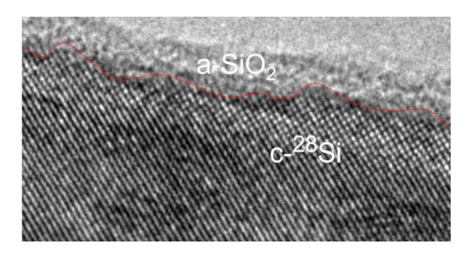
Transmission electron microscope image of silicon-28 nanowire with a layer of silicon dioxide on the surface. Credit: Matthew R. Jones and Muhua Sun/Rice University
