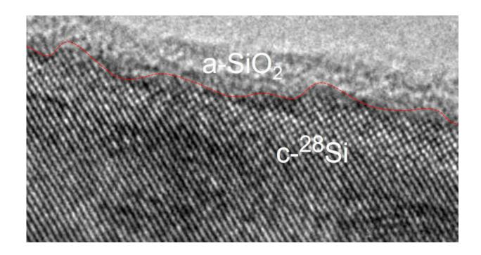
Transmission electron microscope image of silicon-28 nanowire with a layer of silicon dioxide on the surface. Credit: Matthew R. Jones and Muhua Sun/Rice University
