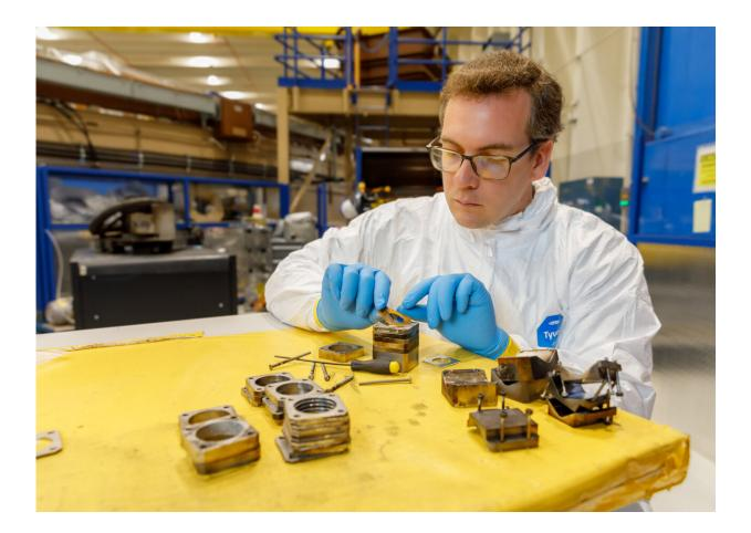
Physicist Chad McCoy at Sandia National Laboratories' Z machine loads sample coatings into holders. When Z fires, researchers will observe how well particular coatings protect objects stacked behind them. Credit: Bret Latter, Sandia National Laboratories
