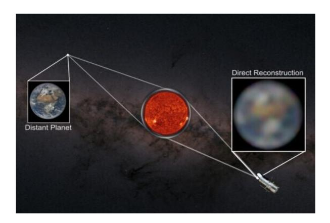
Diagram showing a conceptual imaging technique that uses the sun's gravitational field to magnify light from exoplanets. This would allow for highly advanced reconstructions of what exoplanets look like. Credit: Alexander Madurowicz
