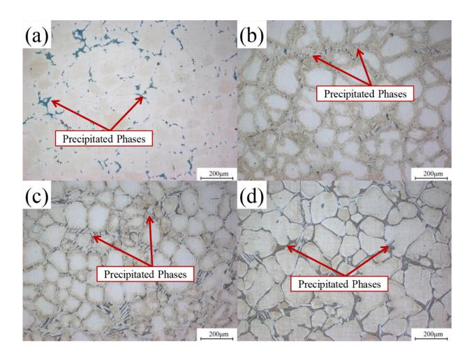
The optical photographs of microstructure for Mg-5Y-1.5Nd-xZn-0.5Zr (x = 0, 2, 4, 6 wt.%) alloys. Credit: *Journal of Magnesium and Alloys* (2022). DOI: 10.1016/j.jma.2022.03.007
