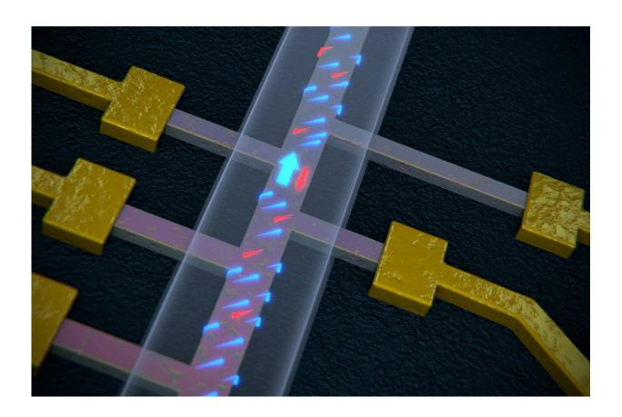
Applying a magnetic field causes current to flow more easily in one direction along the nanowire than in the opposite one. Credit: University of Basel, Department of Physics
