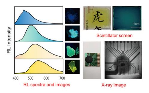
Amorphous polymeric scintillators that exhibit multiple radioluminescence colors will contribute to high-resolution X-ray imaging. Credit: Wei et al., doi 10.1117/1.AP.4.3.035002.
