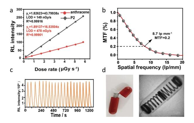
Amorphous polymeric scintillators with multicolor radioluminescence. (a) Behaviors of P2 and anthracene under low-dose-rate X-ray excitation. (b) MTF curves of P2 scintillator screen. (c) The photostability of P2 at 510 nm for continuous X-ray irradiation dosage of 27.35 Gy. (d) Bright field and X-ray images of a metallic spring in capsule using P2 scintillator screen. Credit: Wei et al., doi 10.1117/1.AP.4.3.035002.
