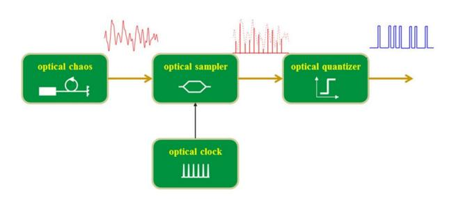
Ultrafast physical random bits can be generated in real time by combining broadband photonic entropy sources with all-optical signal processing techniques. Credit: Pu Li @TUT and GUT.
