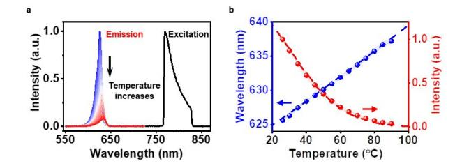
(a) Spectra of the excitation and the upconverted photoluminescence (PL) emission at varied temperatures (25–90 °C). (b) Calculated (dash line) and measured (dots) peak wavelength and PL intensity of the upconverted red emission as a function of temperature, and the shaded range represents the standard deviation measured among 10 samples. Credit: He Ding, Guoqing Lv, Xue Cai, Junyu Chen, Ziyi Cheng, Yanxiu Peng, Guo Tang, Zhao Shi, Yang Xie, Xin Fu, Lan Yin, Jian Yang, Yongtian Wang, Xing Sheng
