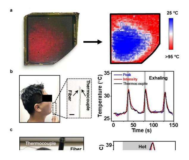
(a) Spatially resolved PL responses of a device array under nonuniform heating (left) and the corresponding temperature mapping (right). (b) Left: Photograph of the exhaling temperature detection with the fiber sensor. Right: Dynamic temperature signals during cycled exhaling activities obtained by the fiber sensor based on the emission peak wavelength shifts and PL intensity changes,
