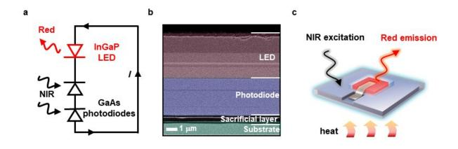
(a) Circuit diagram and (b) Scanning electron microscopic (SEM) image of the optoelectronic upconversion design, including an InGaP red LED and a GaAs double junction photodiode with serial connection. (c) Schematic diagram of the upconversion device for temperature sensing. Credit: He Ding, Guoqing Lv, Xue Cai, Junyu Chen, Ziyi Cheng, Yanxiu Peng, Guo Tang, Zhao Shi, Yang Xie, Xin Fu, Lan Yin, Jian Yang, Yongtian Wang, Xing Sheng
